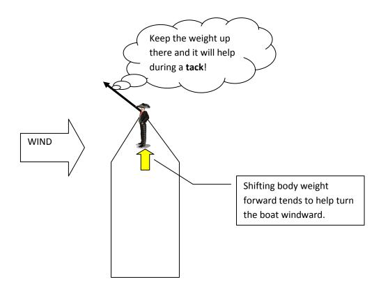
Since these forward/aft weight shifts are smaller, I recommend focusing on lateral weight shifts first while learning rudderless sailing.
