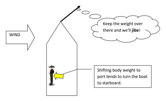
Similarly, shifting your weight to starboard will tend to make the boat turn toward port. Exploit this fact to do a turn in the opposite direction.
