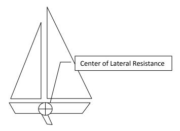
Raising the center board moves the center of lateral resistance back on the boat:
