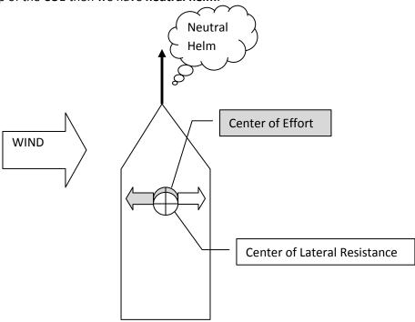
When sailing rudderless in a straight line, we try to keep the <u>COE on top of the CLR</u>.
