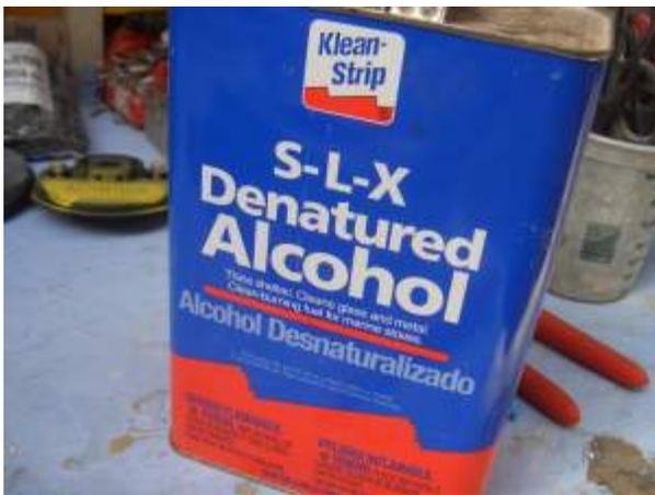
Now get out the alcohol and a clean rag. You've got to clean off the grease (sunscreen in the water) from the board's surface before you start, or the repair may not stick.
