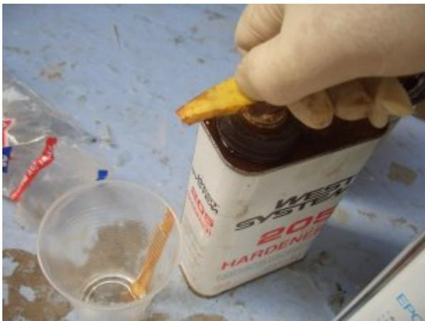
One squirt of resin, and one squirt of hardener provides about two tablespoonfuls of mixed resin/hardener, which is way more than enough for a ding repair.
