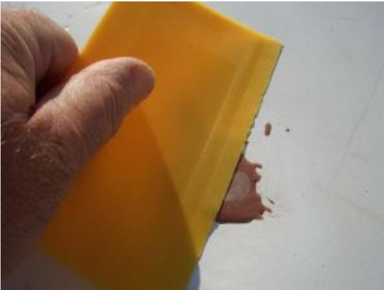
Force the resin/hardener/filler mix into the ding with a yellow plastic squeegee. Once the ding is filled, use the squeegee to level off the top of the mix, leaving a smooth surface.
