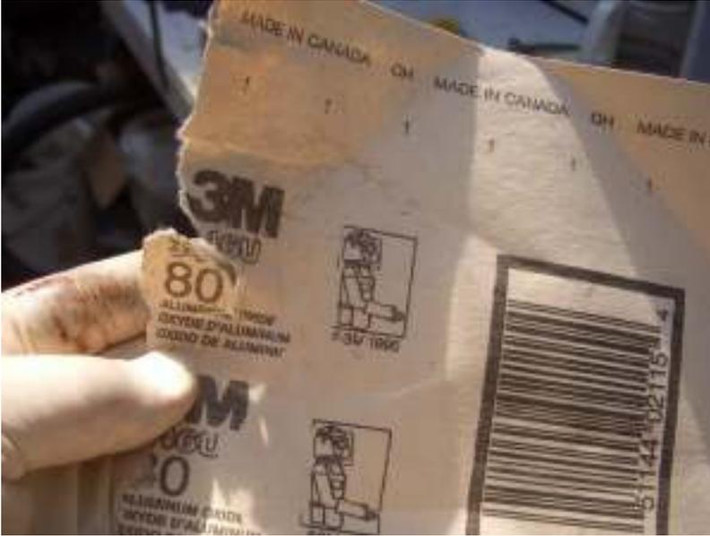
Find a sheet of clean sandpaper. This is 80 grit, which will sand the board's surface to a very rough texture, which is better for the repair.
