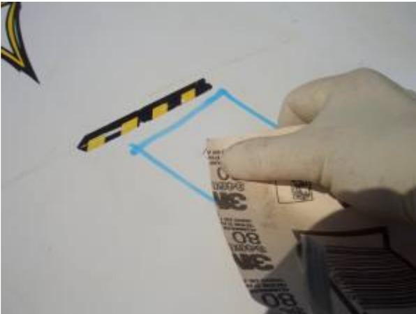
Sand an area about 1" around the hole, just to roughen the surface. Don't sand all the way through the board surface, just roughen it.
